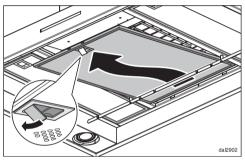
Open the grease filter lock, lower the grease filter slightly, unhook it at the back, and remove.
